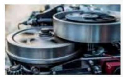
Counter-rotating crankshafts in the powerhead reduce noise and vibration to a minimum.
