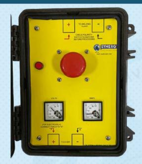
Once the cables from the welding power-source are connected, turn on the machine and check to see that the volt meter registers (no need to connect the welding cables to the diver yet). The volt meter is a zero centred meter and so the needle should rise in an upwards direction. If the meter falls (drops) in a downward direction, then the cables are not matched like-for-like! (Check connections and/or polarity switch and re-test).
