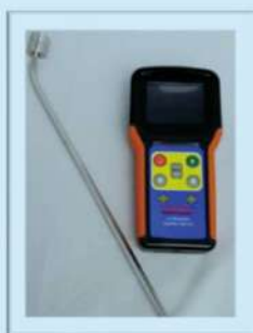
Probe with Ultrasonic meter
